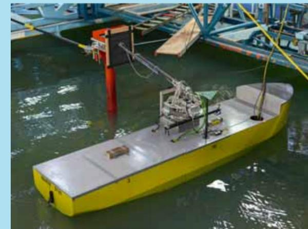
Seaqualizer, spring balanced offshore access bridge
