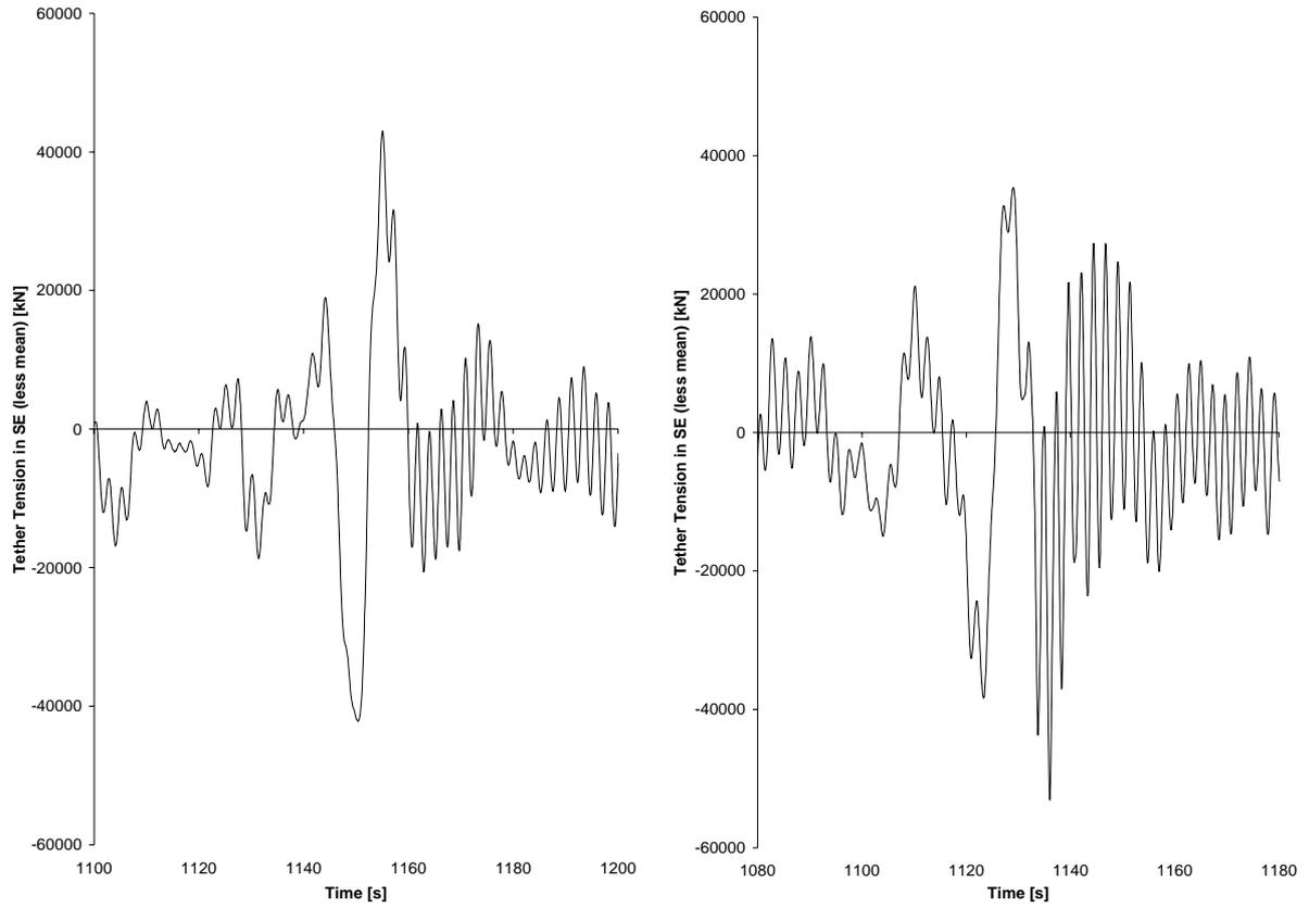
**Figure 10 Governing 100 year (left) and 10 000 year (right) negative tension excursions in SE tether**
