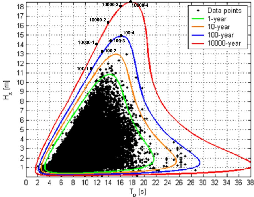
**Figure 5** Contours of Significant Wave Height and Spectral Peak Period for the Snorre Field (From Ref./4/)
