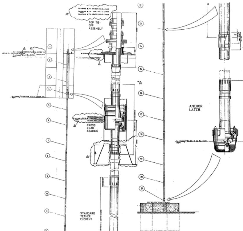
**Figure 4 Overview of Snorre A tether system: top connection left and bottom connection right (note that dimensions are preliminary)**
