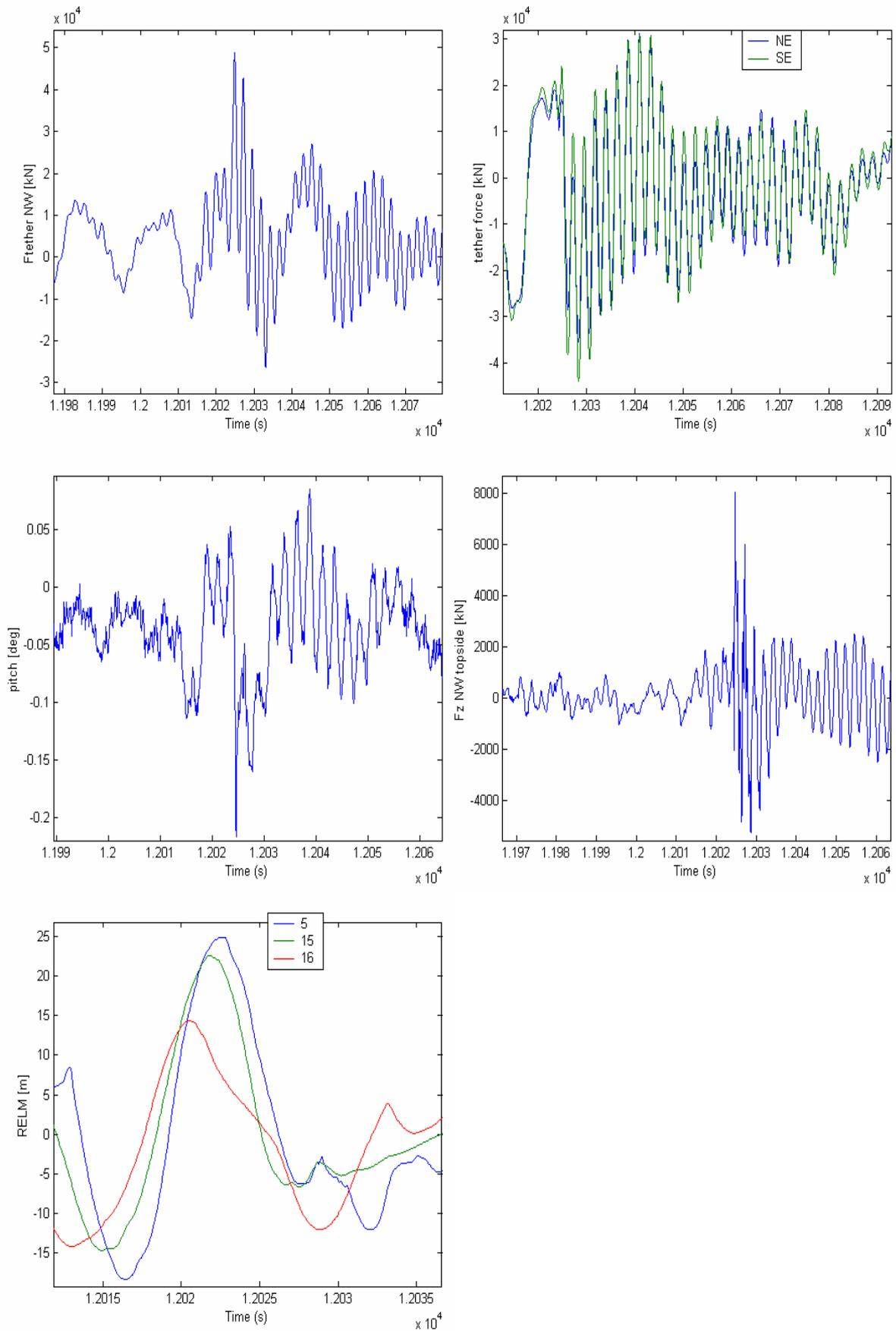
**Figure 12 Measurements of Extreme Event (Seastate 10 000-4 from W)**
