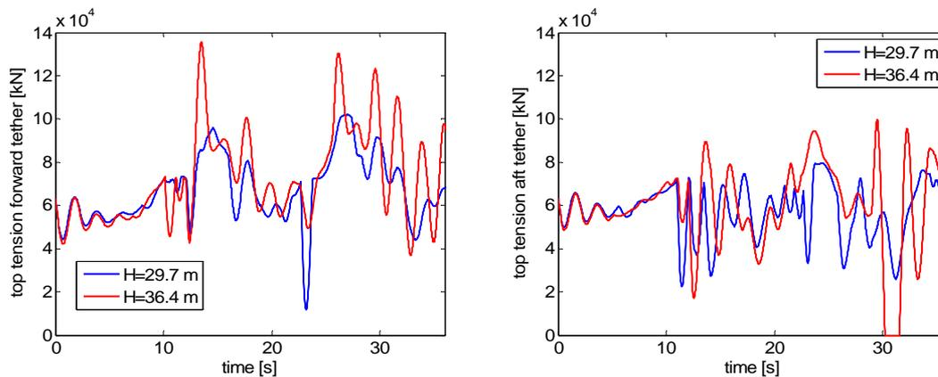
**Figure 17 Tether Tension Timeseries**
