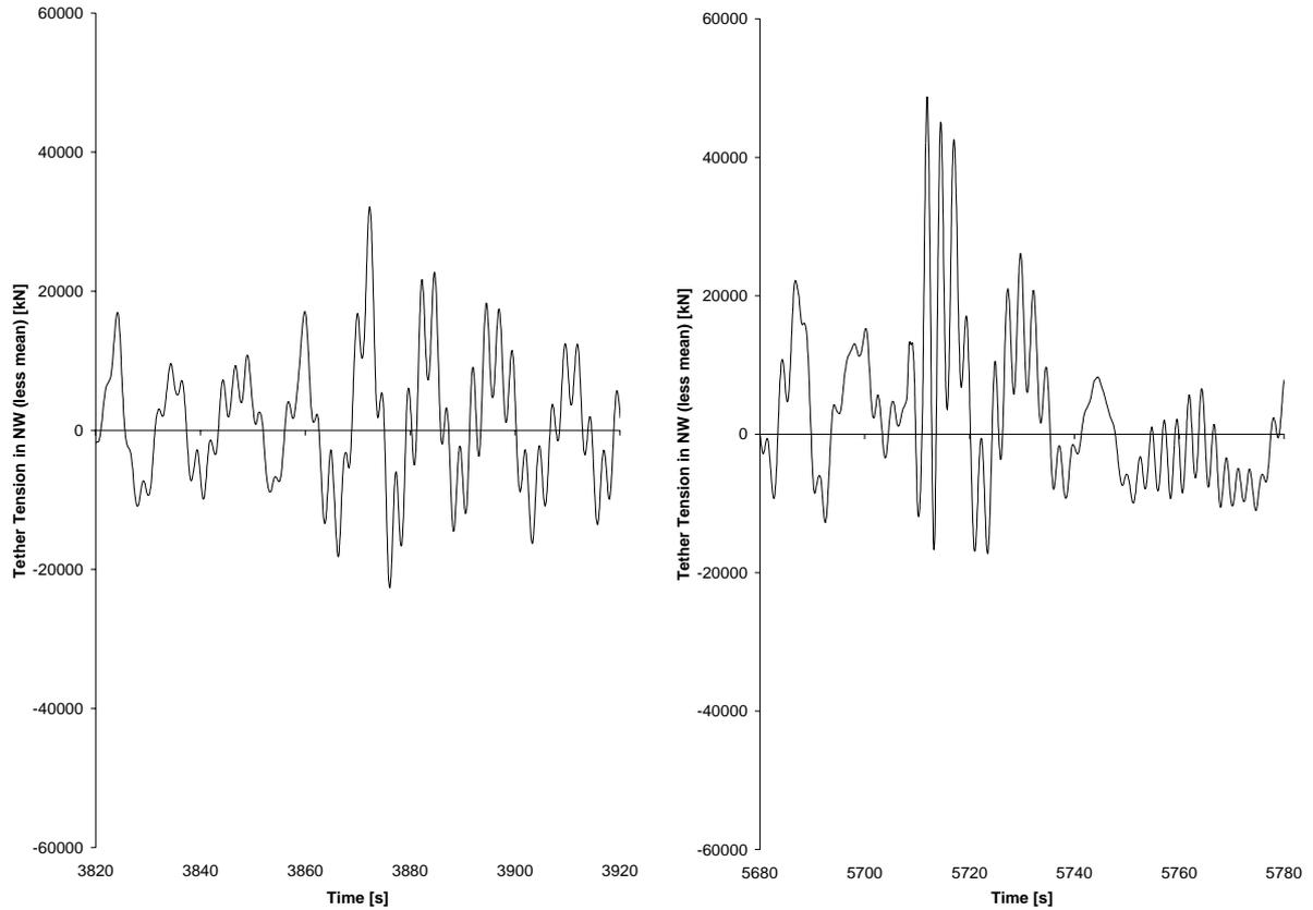
**Figure 11 Governing 100 year (left) and 10 000 year (right) positive tension excursions in NW tether**
