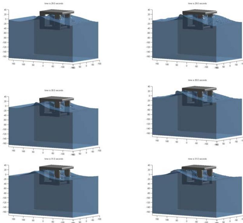
**Figure 16 Snapshots during iVOF Simulation (largest wave right)**
