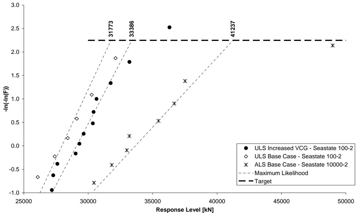
**Figure 9 Measured Maximum deviations from mean tension in NW corner with all weather from NW**
