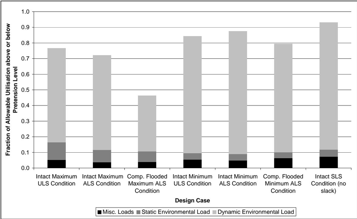
Figure 19 Tether Utilisation for the Different Design Cases
